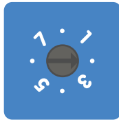
Rotary switch set to position 2
